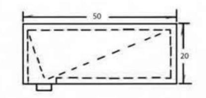
Drainage Slope Of 1/2 Inch Per Foot
